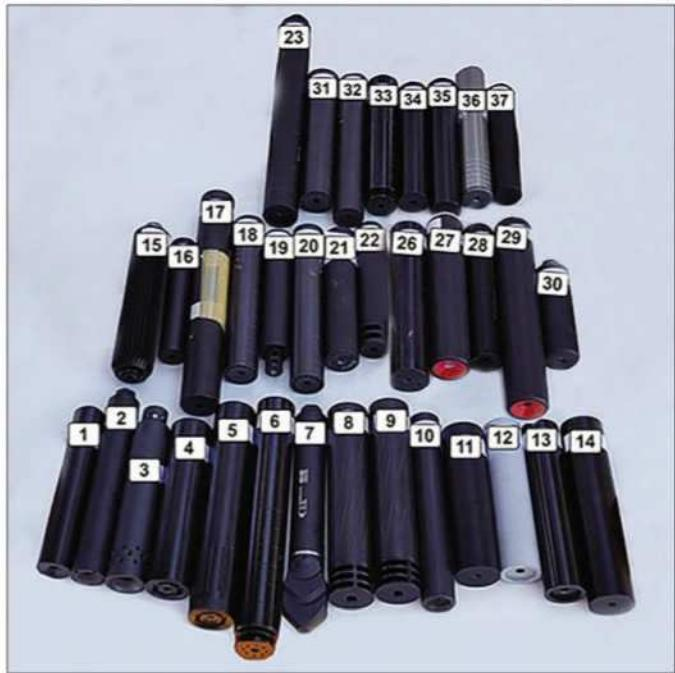
The silencers that had been entered for the demonstration/test. Use the table on the immediate right to match the numbers and identify the products. Products 38, 39 and 40 are not in the photo because they were entered after the picture was taken.
