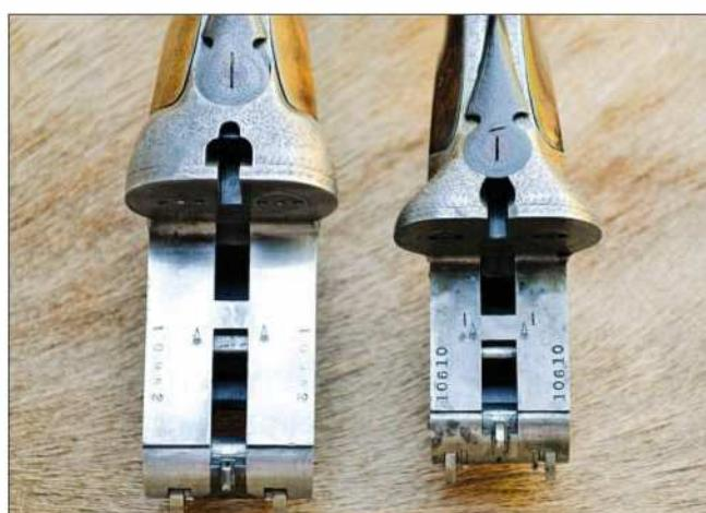
An interesting view of a PHV-1 action (**left**) made for a .470 NE double rifle and a screw-grip action for a 20-bore shotgun (**right**). Note the differences in the cut-outs required for the two rib extensions. Both of these examples date from 1914 and both bear the name of the London gunmaker William Evans.
