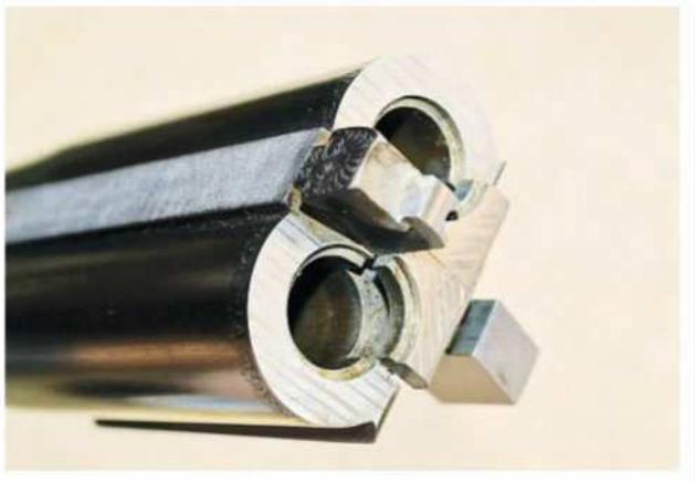
The screw-grip rib extension consists of a spade-shaped rib extension (**top**) that was wedged into place by the threaded top-lever spindle (**bottom**) that cammed the barrels down and into place.
