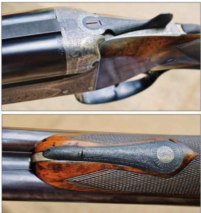
**TOP AND BOTTOM:** Top-grade Webley & Scott-made double guns and rifles were very well made, as the workmanship on this .360 No 2 NE double rifle bearing the name of George Gibbs of Bristol shows. Note the elegant lever keeping the fore-end in place, the intercepting sears of the action, fine engraving, and excellent fit and finish throughout.
